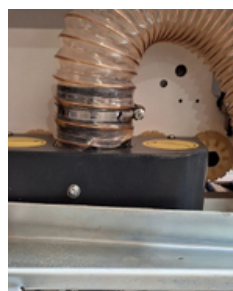
Pre-milling unit two HF motors
