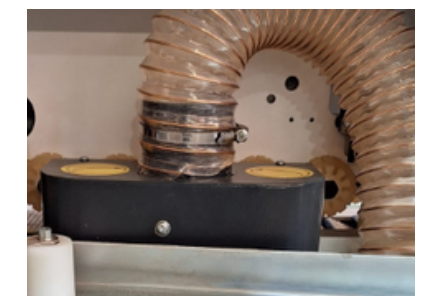
Pre-milling unit with two HF motors included
